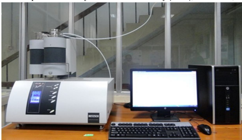
Figure 2. Thermogravimetric Analysis Machine (STA 449 F3 Jupiter)
