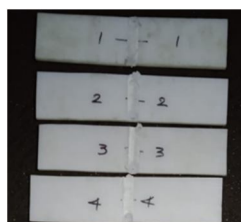
Fig: 6 After FSW of UHMWPE Plates
