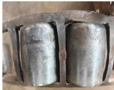
Figure-4: Cage Fracture at Bearing NDE
