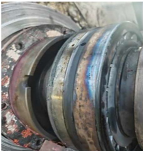
Figure-3: bearing color change due high temp.
