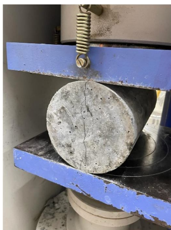
Fig 1.6 Performing Split Tensile Testing
