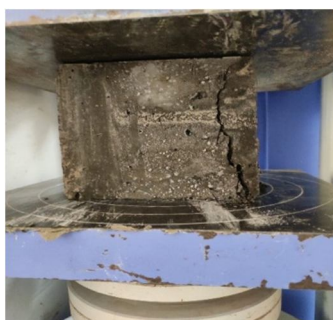
Fig 1.6 Performing Compression Testing
