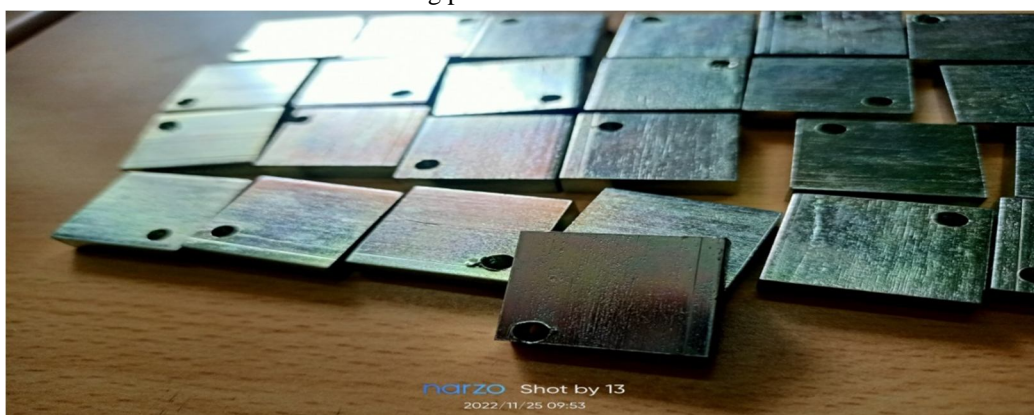
Figure 2. Specimen after zinc plating
