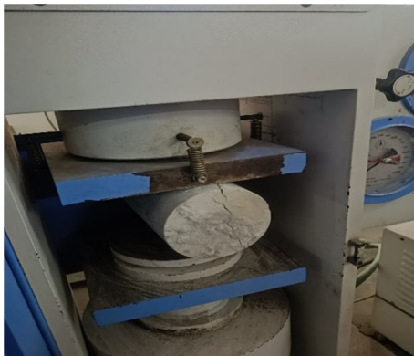
Fig5&6: Compressive strength test
