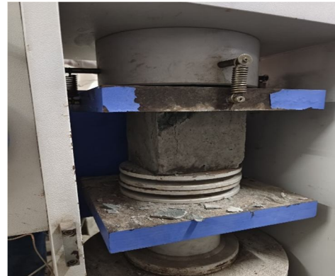
Fig5&6: Compressive strength test
