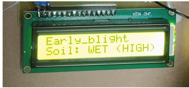
Fig 6: LCD Display Output Showing Disease Detection and Soil Status
