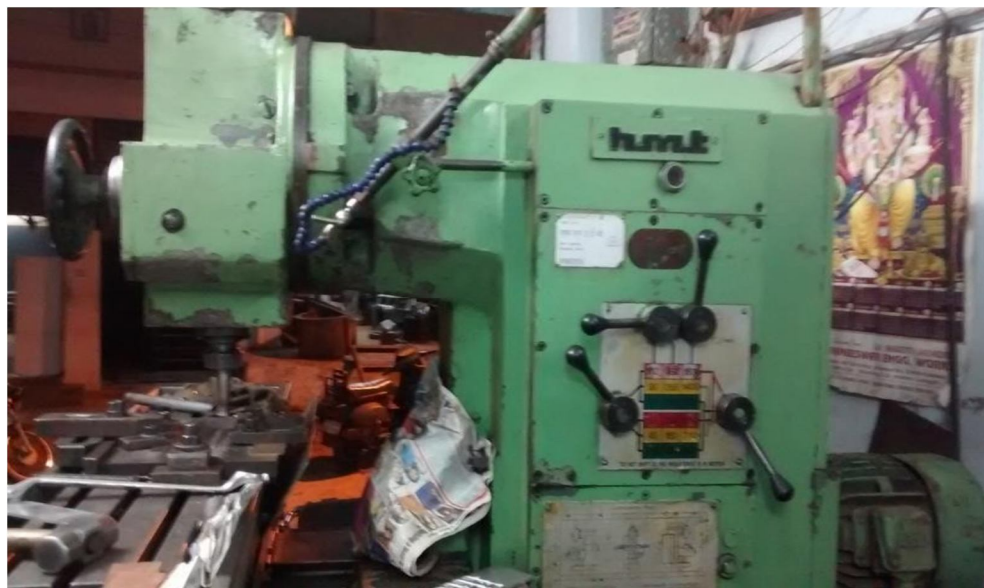
Machine used for Friction Stir Welding
