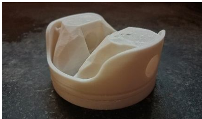
Figure 8 3d printed prototype of the piston
