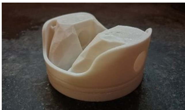
Figure 8 3d printed prototype of the piston
