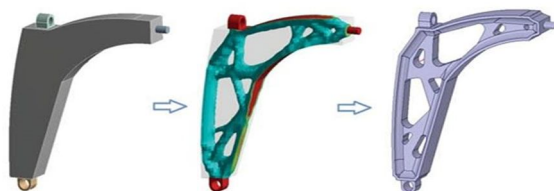
Figure 2: Topology optimization example
