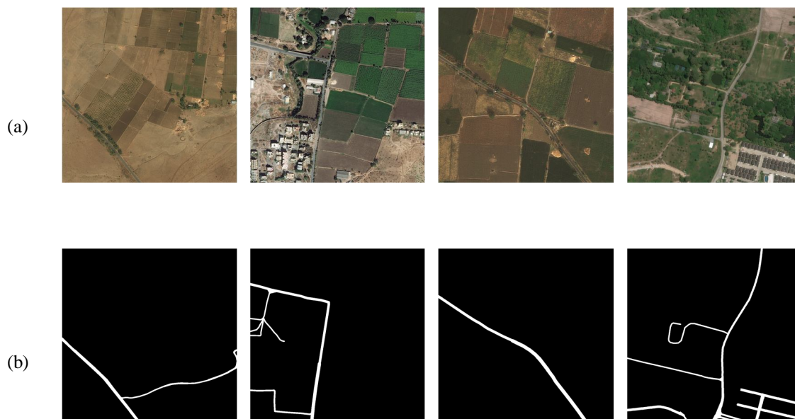
Fig. 1 Sample images from the dataset: (a) satellite images and (b) corresponding ground-truth road segmentation masks.
