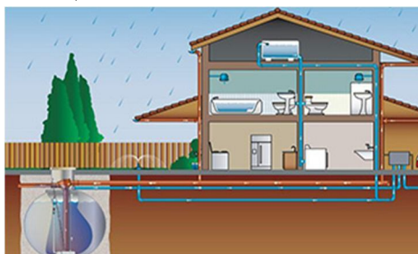
Fig. 1 Rain water harvesting
