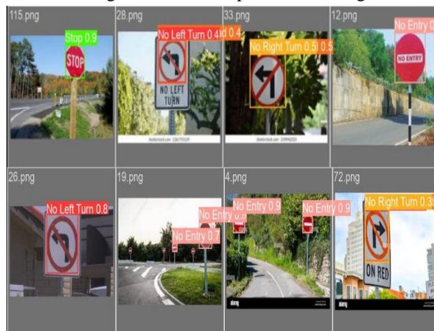
Fig. 5. Validation images containing prediction labels and mAP
