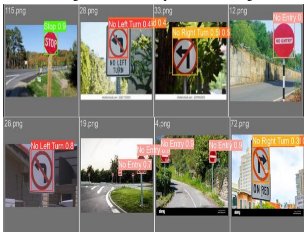
Fig. 5. Validation images containing prediction labels and mAP
