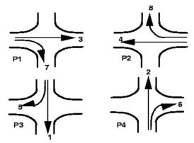
Third possible way of providing Four-phase signal
