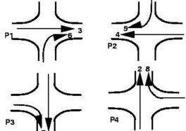
One possible way of providing Four-phase signal
