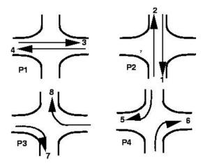
Second possible way of providing Four-phase signal
