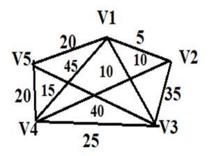
$$\begin{split} & \text{Start with } V_1, \, V_2 \text{ is nearest.} \\ & \text{Cycle } C_2 = V_1 \, V_2 \, V_1 = 0 \\ & V_1 \, V_2 \, V_3 \, V_1 = 5 + 35 + 10 = 50 \\ & C_3 = V_1 \, V_2 \, V_3 \, V_1 \end{split}$$
