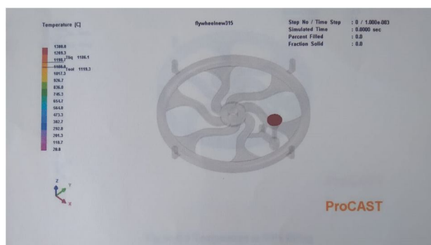
Fig 9: Temperature at 0% filling
