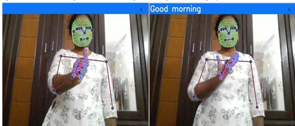
Fig. 6 Sign is detected as Good Morning in real-time
