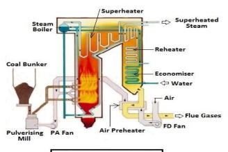
Pulverized Coal-Fired Boiler
