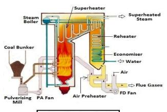
Pulverized Coal-Fired Boiler
