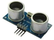
The HC-SR04 ultrasonic sensor uses sonar to determine distance to an object like bats or dolphins do. It offers excellent non-contact range detection with high accuracy and stable readings in an easy-to-use package. From 2cm to 400 cm or 1" to 13 feet. Its operation is not affected by sunlight or black material like Sharp rangefinders are (although acoustically soft materials like cloth can be difficult to detect). It comes complete with ultrasonic transmitter and receiver module.
