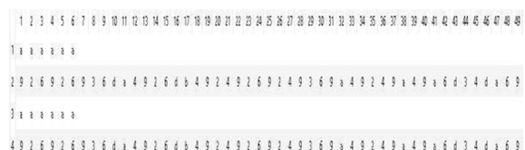
Figure 6 - Demodulated hexadecimal key fob message
