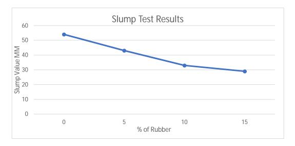
The above fig shows the slump results. It was observed that, the slumps decreased as the rubber content were increased in the mix. It was a Low Slump (25 - 50 mm). It was suitable for Low Workability mixes used for foundations with light reinforcement. Roads vibrated by hand operated machines.
