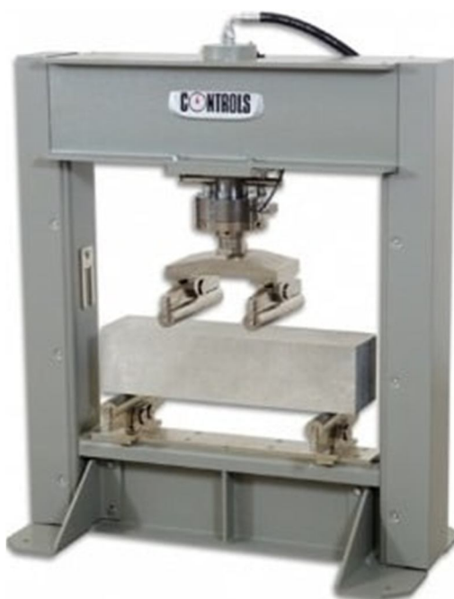
Fig.3.5: Flexural Test Machine and Concrete Specimen (ASTM C78)
