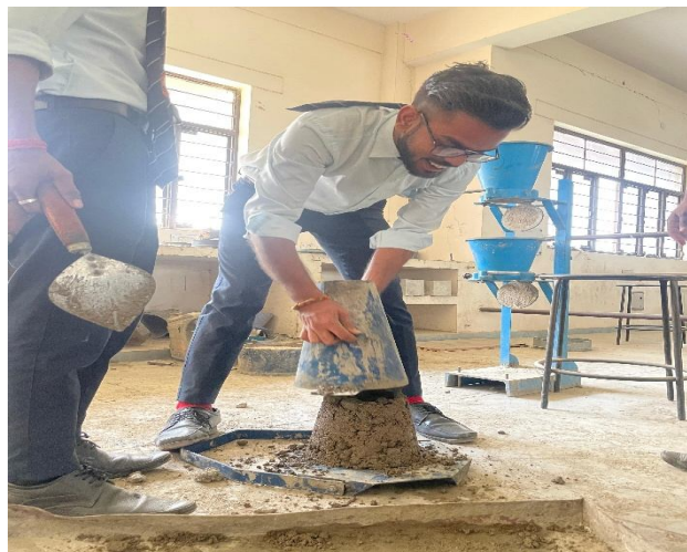
Slump Cone Test
