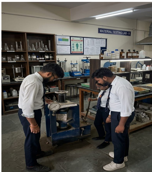
Compressive Strength Test
