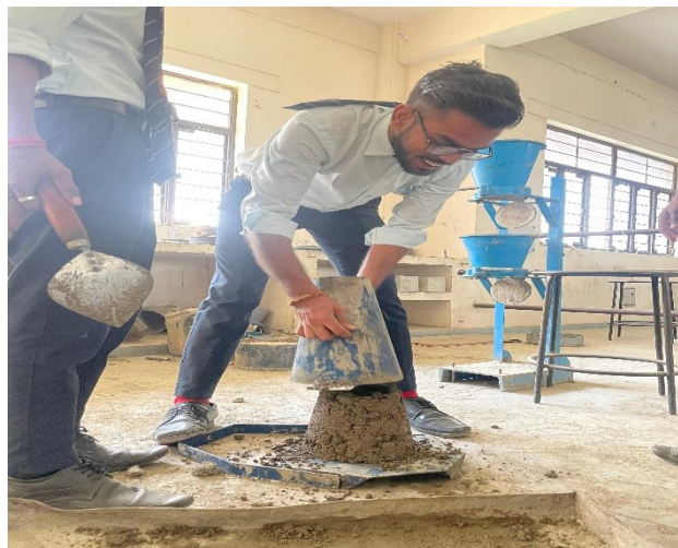
Slump Cone Test
