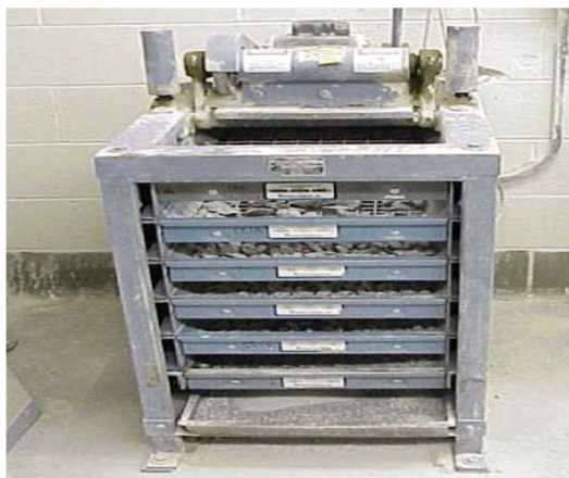
Fig 4.4 Sieve Shaker for coarse aggregates
