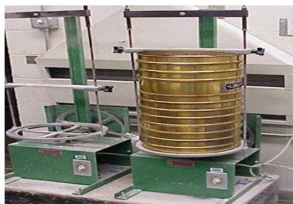
Fig 4.2 : Sieve Shaker for fine aggregates
