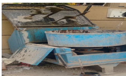
Fig 4.6 Concrete Mixer (Pan type)
