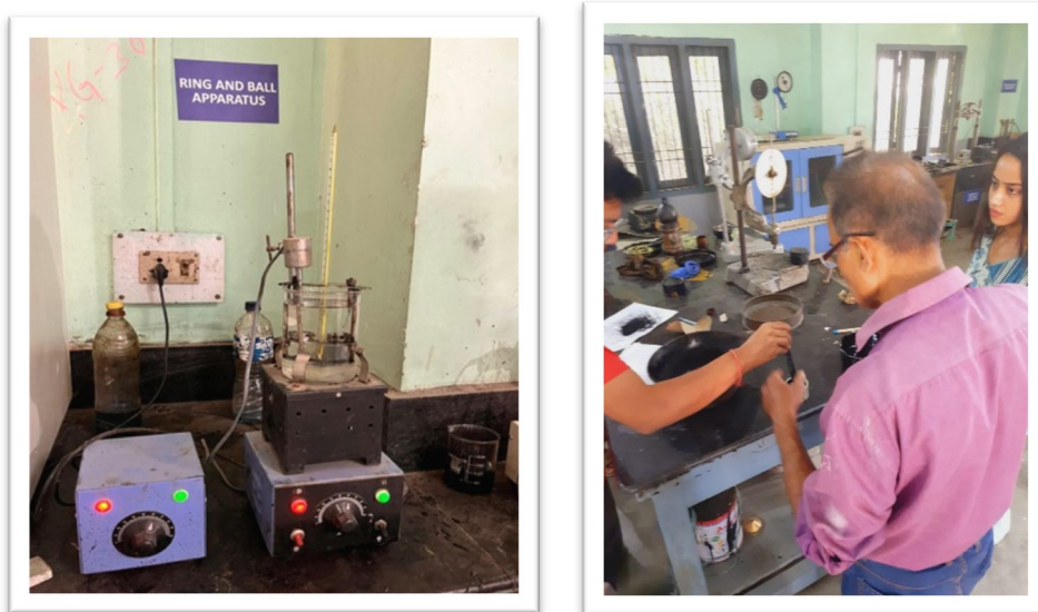
Fig. 4 Standard Test Method For softening point of bitumen
