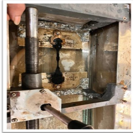
Fig. 6 Standard Test Method For ductility of bituminous materials
