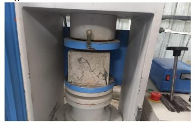
The compressive strength is decreased with an increase in the percentage of the tyre rubber chips. The results of compressive strength of cubes for 7 days and 28 days. The concrete mix was prepared with water-cement ratio of 0.55 then accordingly. The concrete cubes are casted. The same cubes are cured in water curing tank in laboratory at normal room temperature and are tested at 7th and 28th days with the help of Compression Testing Machine.
