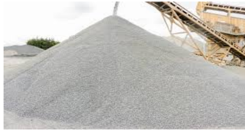
Fig 2: Stone/Quarry dust Aggregate
