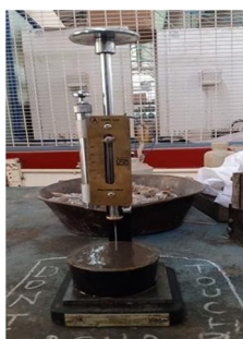
Fig 5.2 Initial Setting time of Cement
