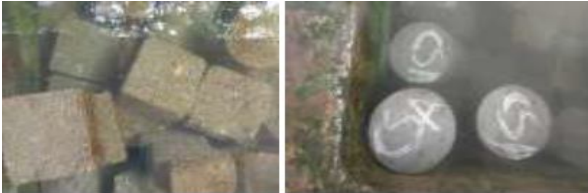
Fig 4.3 :-Curing of cubes and cylinders
