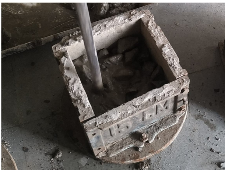
Fig. 7 Mixing & Tamping concrete in layers by tamping rod
