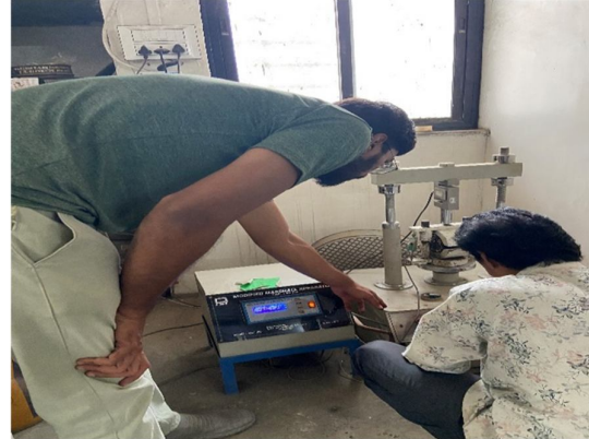
Marshall Stability Test
