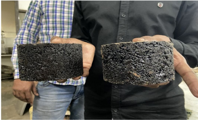
Diff between BC mold with & without plastic
