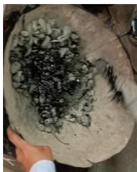
Fig-4: Mixing of Bitumen
