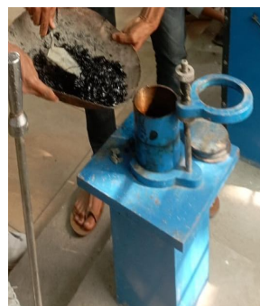
Fig-5: Fill Mix Bitumen in mould
