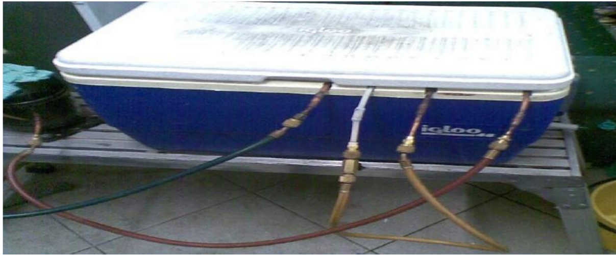
Figure no: 1 Refrigeration Evaporator
