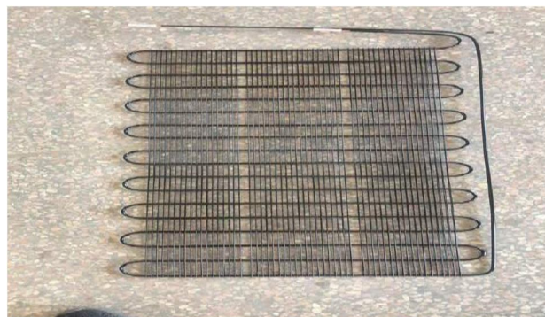
Figure no.3: Condenser
