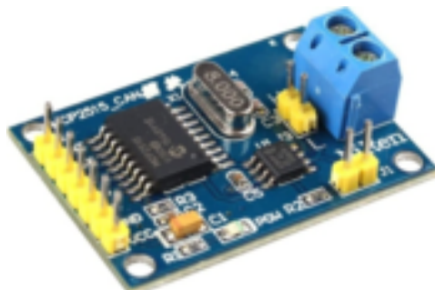
Figure 6: MCP2515 CAN Communication Module
