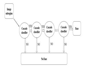
When the subregion is applied as input to first classifier it checks for the presence of face features if it is detected to be face, the output is treated as 'maybe' (true) and this subregion is applied as input to next classifier. If the classifier does not detect the face then the output is 'no' (false) and the subregion is discarded.
