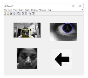
3) Eye balls facing towards right: If the direction of eye balls is detected to look right side then it is indicated by right arrow.
