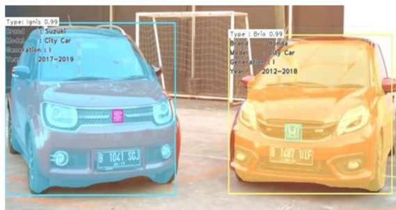
Fig.6: Detection result of non-identical cars obtained from the modified Mask R-CNN algorithm [7]
