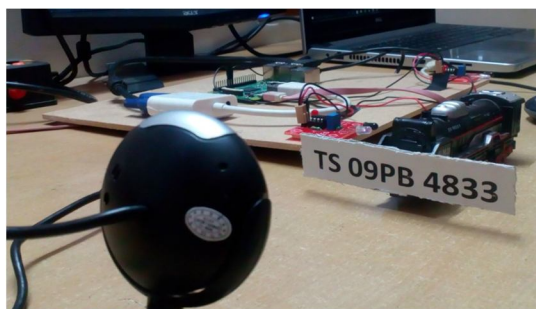
Fig. 7 Image of the number plate being captured by camera
