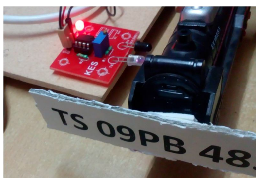
Fig. 5 Blinking of LED present on second IR sensor
