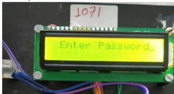
Fig: 3 Display Enter password for unlocking car
