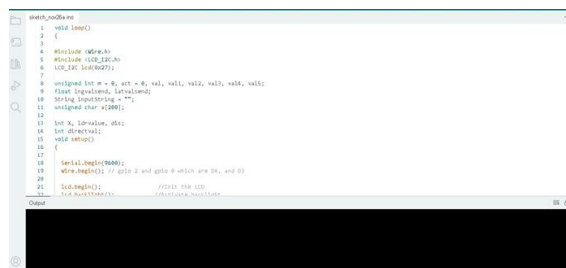
FIG 4: Integration of LCD display and LIFI Receiver with ESP8266 NODE MCU WIFI DEVELOPMENT BOARD
