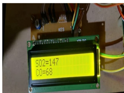
Fig.8: Displaying sensor value on LCD
