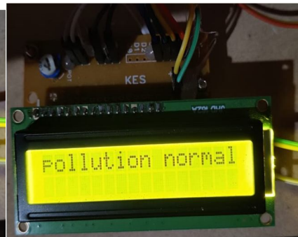
Fig.7: Displaying pollution condition on LCD
