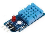
Fig 2 Diagram for DHT11
