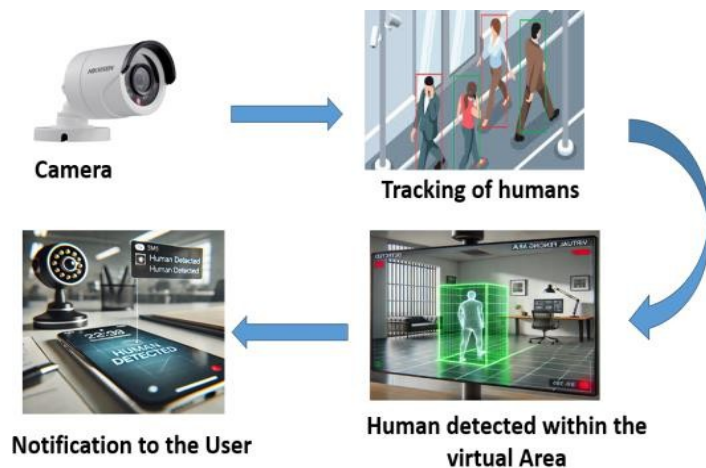
Figure 1 Block diagram of the virtual fencing area
