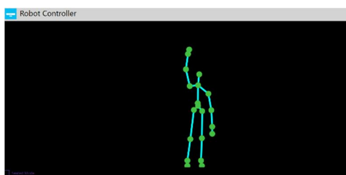
Figure 5: Gesture for robot to move left
