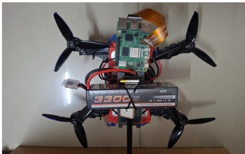
Fig. 7: Assembled drone platform with onboard electronics.
