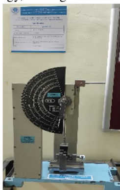
Fig 3. Impact testing machine
