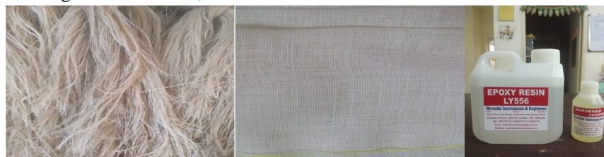
Fig.1a Raw banana fiber Fig.1b Woven BD banana fiber Fig.1c Epoxy Resin and Hardener
