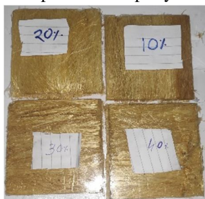
Fig 2. Banana fiber reinforced epoxy composite
