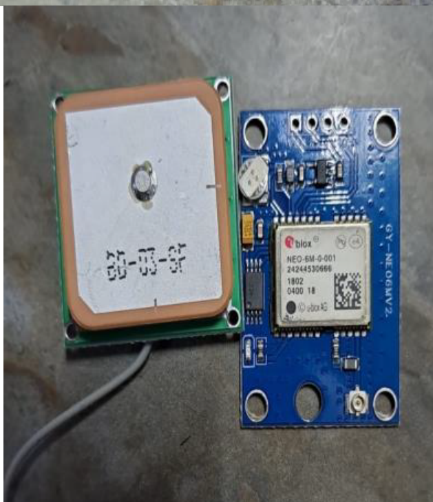
Fig 1. Representing the structure of the drone, Fig 2. Image representing the sim module using for the communication between the drone and the operator., Fig 3. Image representing the NEO-6M GPS Module
