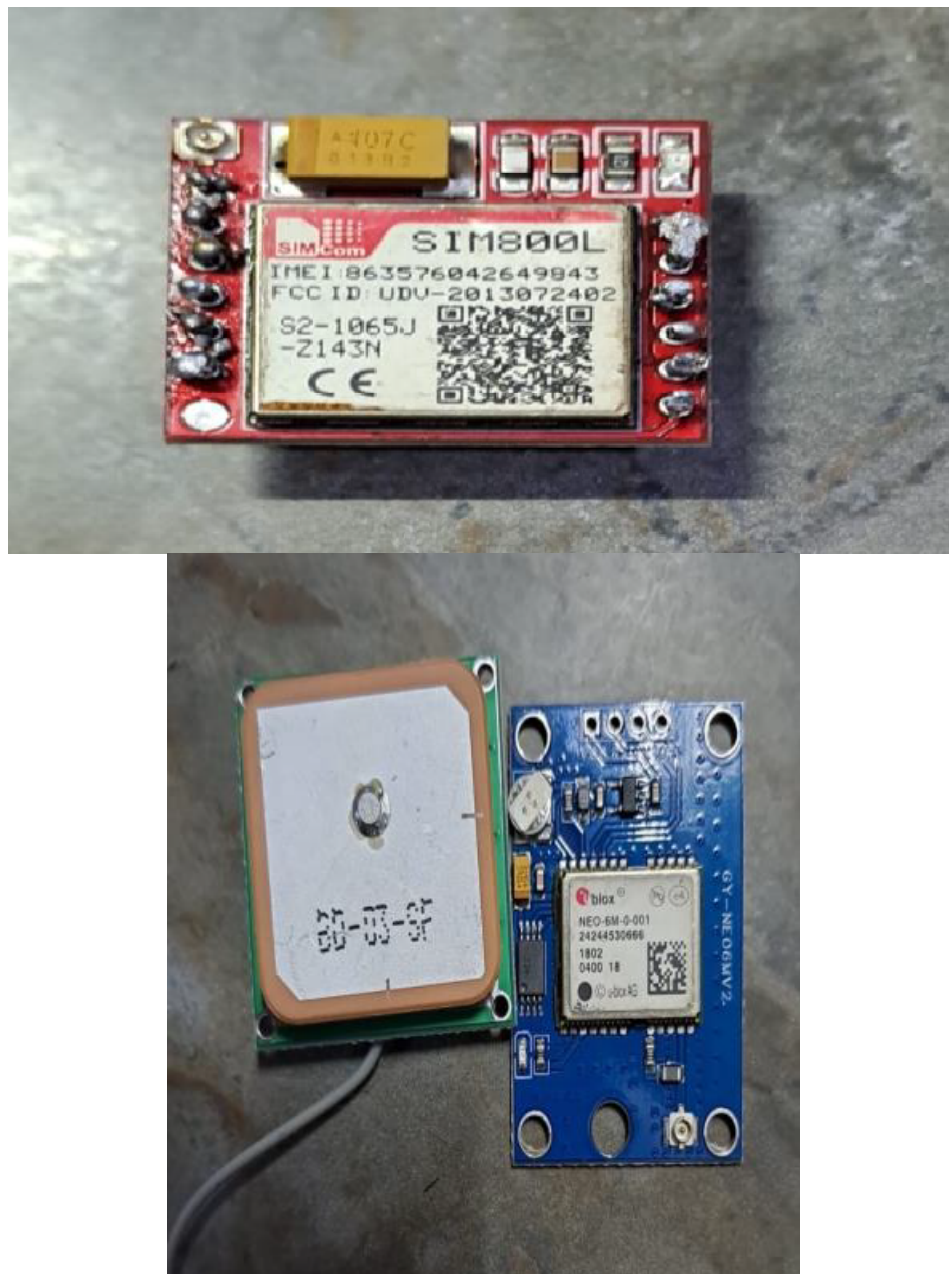
Fig 1. Representing the structure of the drone, Fig 2. Image representing the sim module using for the communication between the drone and the operator., Fig 3. Image representing the NEO-6M GPS Module
