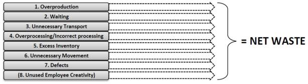
In addition, when examining a process with the aim to detect waste and eliminate these, activities need to be classified in some way. Monden (1993) identified three different types of operations in an internal manufacturing context. The activities could be:
