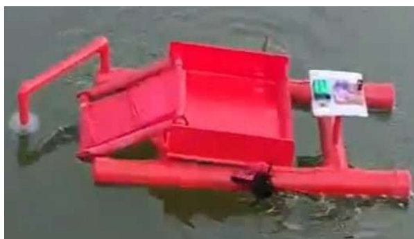
Fig. 1. Model of Water Hyacinth Remover
