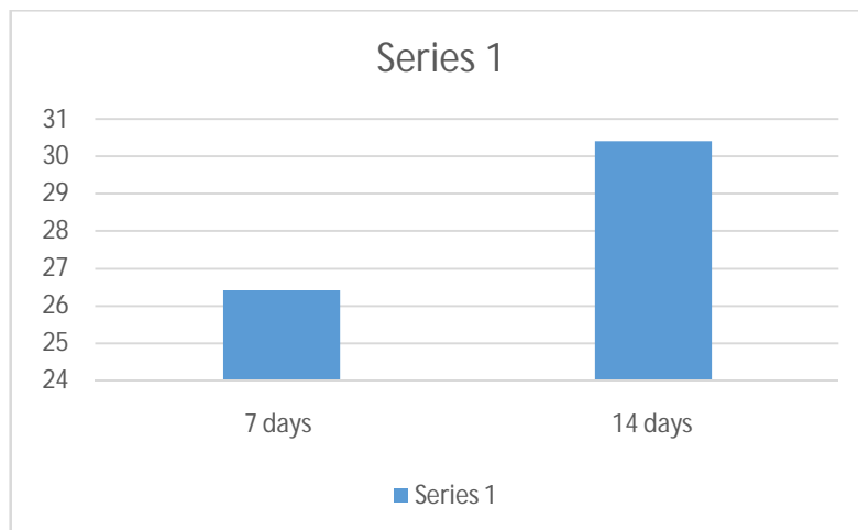
Compressive strength of permeable concrete cube
