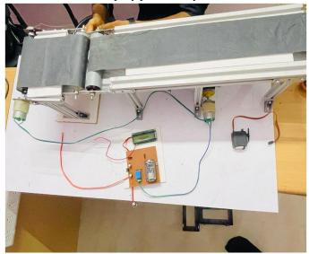
We are working for the issue and have to give one small demo prototype as per the company requirements. Here we are using load cell to measure the weight, for demo 100gms soap are accepted and below that are rejected. The servo motor use to rotate the selector plate after the conveyor belt for selected and rejected. The data of counting is sent to the cloud server as well as the conveyor motor start and stop time we can monitor online.
